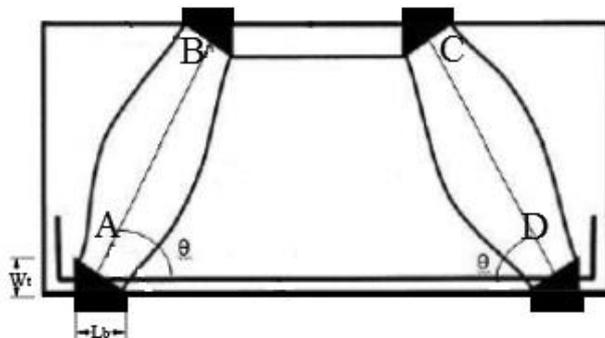
Fig. 11 Typical STM for deep beam
