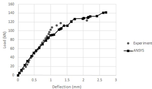
Fig. 6 Load Deflection Plot for Beam E1
