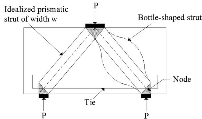
Fig. 1 STM for deep beam with central point load
