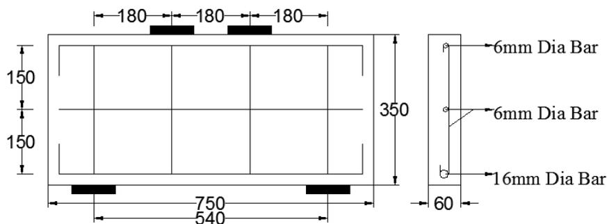
Fig. 4 Typical reinforcement details of deep beam
