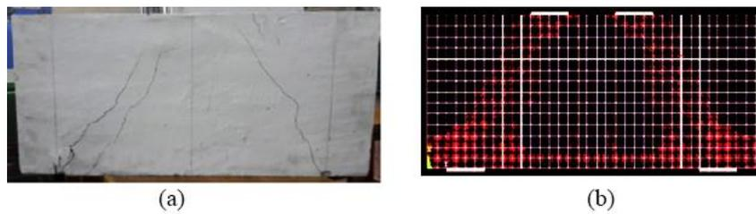
Fig. 10 Crack pattern for beam E1 (a) From Experiment (b) From ANSYS
