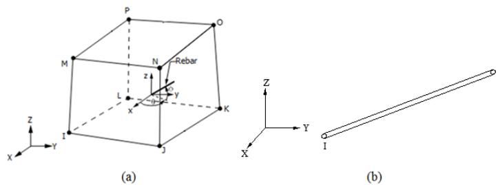
Fig. 2 Solid65 element and Link180 element
