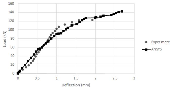
Fig. 7 Load Deflection Plot for Beam E2
