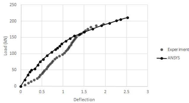
Fig. 8 Load deflection plot for beam E3
