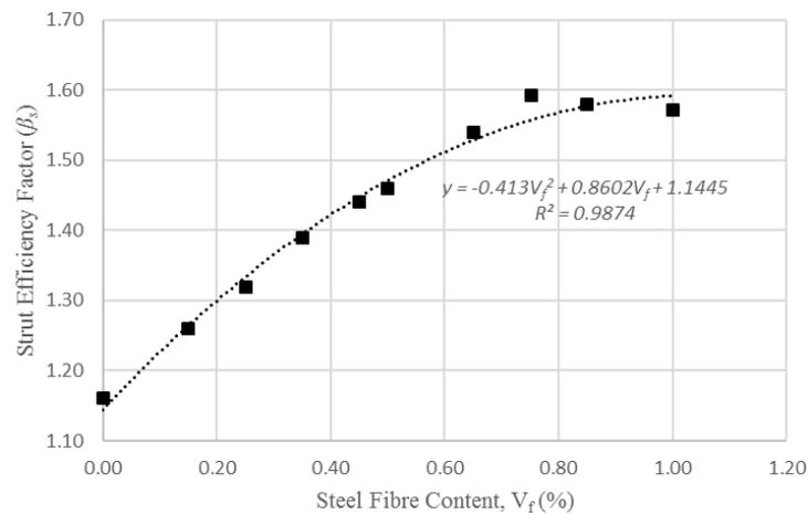
Fig. 12 Plot showing variation of efficiency factor with steel fibre ratio
