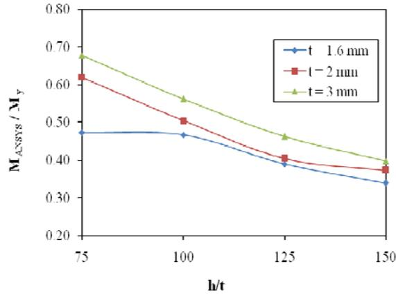
Fig. 9 Effect of section depth and thickness variation
