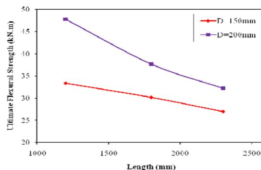
Fig. 5 Effect of length variation of stiffened cold-formed steel built-up open section
