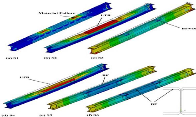
Fig. 4 Failure pattern on effect of bearing plate and stiffener at support and loading point
