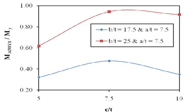
Fig. 11 Effect of variation in flange width
