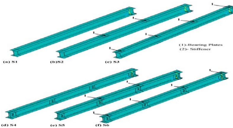
Fig. 3 Model of bearing plate and stiffener-cold-formed steel built-up open section
