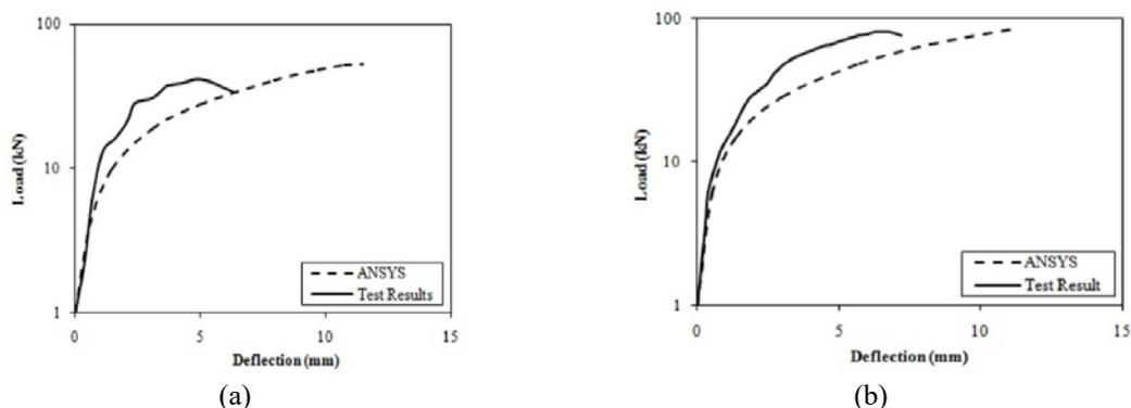
Fig. 7 Load-Deflection curve (a) USB-2 (b) SB-2
