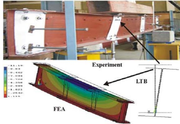
Fig. 8 Lateral torsional buckling failure of the specimen -USB-3
