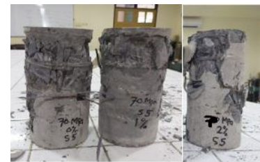
Specimen f_c' = 70.5 MPa, hoop spaced = 50 mm
