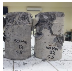
Specimen f_c' = 50.6 MPa, hoop spaced = 50 mm
