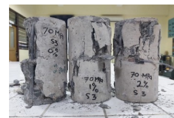
Specimen f_c' = 70.5 MPa, hoop spaced = 100 mm
