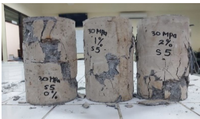
Specimen f_c' = 34.5 MPa, hoop spaced = 50 mm
