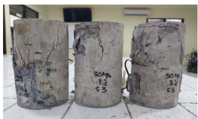
Specimen f_c' = 34.5 MPa, hoop spaced = 100 mm
