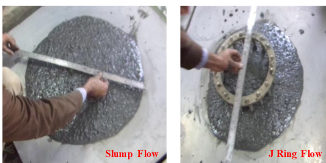
Fig. 8 Observation of slump flow and J Ring flow tests
