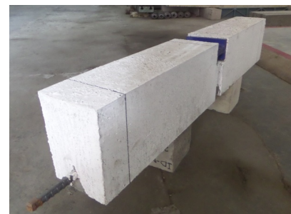
Fig. 4 Test specimen for pull-out test
