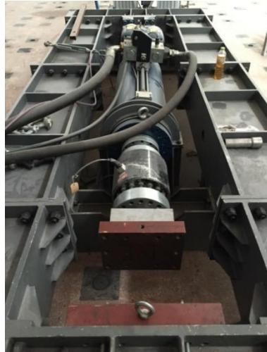
(a) Electric-hydraulic servo multi-function testing machine
