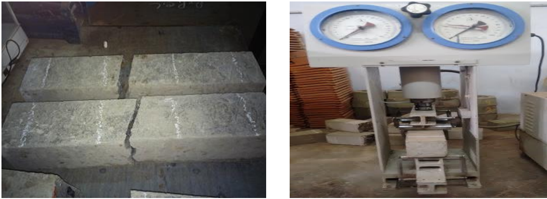
Fig. 13 Flexural Strength arrangement and cracked beams
