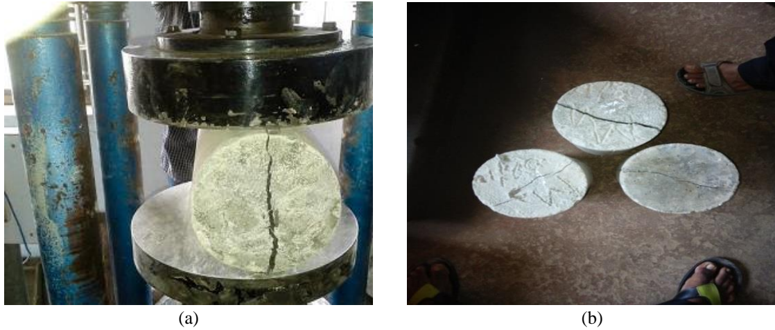
Fig. 11 Arrangement for split tensile strength and cracked cylinders
