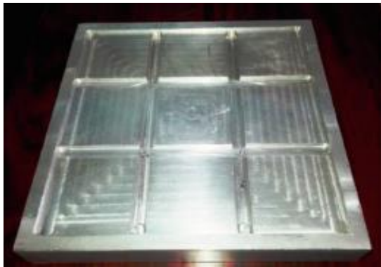
(a) The aluminum mold (200×200 mm)
