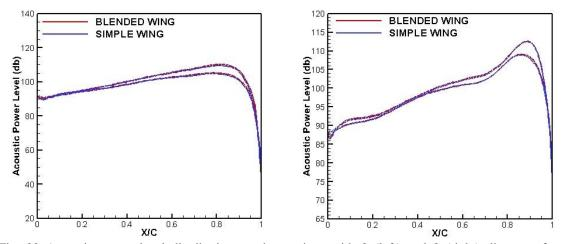
Fig. 22 Acoustic power level distribution on the sections with 2 (left) and 8 (right) distances from symmetry plane
