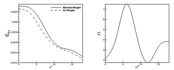
Fig. 15 Skin friction CD (left) and difference (%) (right) versus angle of attack for simple and blended Wings
