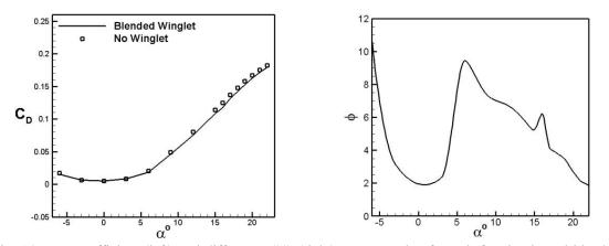
Fig. 14 Drag coefficient (left) and difference (%) (right) versus angle of attack for simple and blended wings
