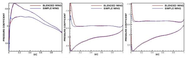
Fig. 11 Comparison of pressure coefficient distribution of simple and blended wings in 15° angle of attack for sections near wing root (left), seco<sup>nd</sup> twist location (middle), and wingtip area (right)
