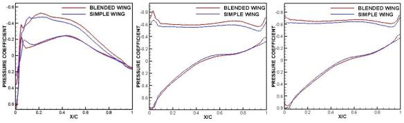
Fig. 12 Comparison of pressure coefficient distribution for simple and blended wings in 20° angle of attack for sections near wing root (left), 2<sup>nd</sup> twist location (middle), and wingtip area (right)
