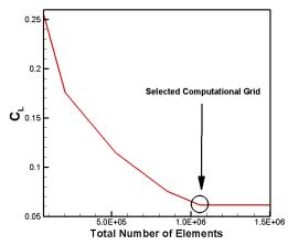
Fig. 8 Changes in lift force coefficient in terms of number of elements and the selected computational grid
