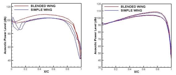
Fig. 23 Acoustic power level distribution on the sections with 12 (left) and 16.8 m (right) distances from symmetry plane
