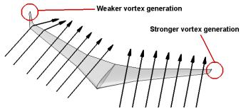
Fig. 3 Main effects of winglet configuration on the streamlines
