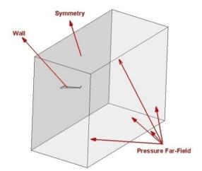
Fig. 7 Defined control volume and applied boundary conditions
