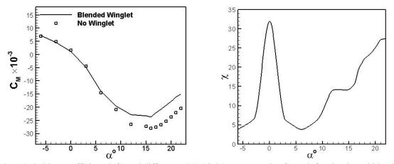
Fig. 16 Pitching coefficient (left) and difference (%) (right) versus angle of attack for simple and blended Wings
