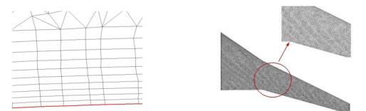
Fig. 6 Computational grid around wing (left) and on the wing surface (right)
