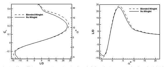
Fig. 17 Lift coefficient versus L/D and angle of attack (left) and L/D versus angle of attack (right) for simple and blended Wings
