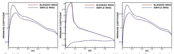
Fig. 10 Comparison of pressure coefficient distribution of simple and blended wings in 0° angle of attack for the section near wing root (left), 2<sup>nd</sup> twist location (middle), and wingtip area (right)
