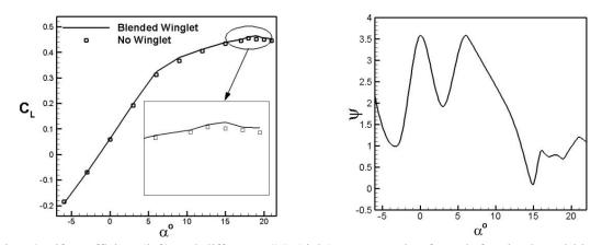
Fig. 13 Lift coefficient (left) and difference (%) (right) versus angle of attack for simple and blended wings
