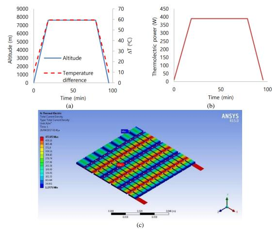
Fig. 2 Results of calculations for the thermoelectric energy profile during a median flight journey of ATR 72 aircraft: (a) altitude and hot-cold temperature difference profiles, (b) total thermoelectric power profile for 29785 HZ-9 TEG modules and (c) results of simulations using ANSYS for a HZ-9 TEG module on ATR 72 at cruise altitude
