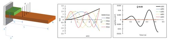
wing with a local load F and a piezoelectric device
