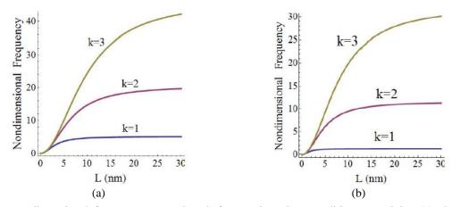
Fig. 5 Nondimensional frequency versus length for two boundary conditions containing (a) clampedclamped and (b) clamped-free with the first three frequency modes for exponential law (nonlocal parameter 1 nm)
