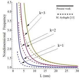
Fig. 2 Nondimensional frequency for clamped-clamped boundary condition
