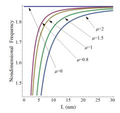
Fig. 10 Nondimensional frequency versus length with regard to different value for nonlocal parameter assumed for clamped-free FG nanobeam for power law
