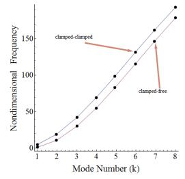
Fig. 15 Nondimensional frequency versus mode number for two boundary conditions demonstrated for exponential law
