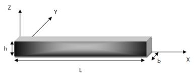
Fig. 1 Schematic illustration of FG nanobeam
