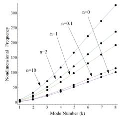
Fig. 13 Nondimensional frequency versus mode number containing different *n* value for clamped-clamped case (power law)
