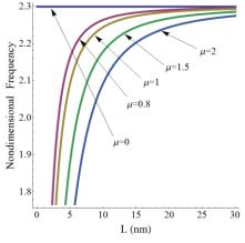
Fig. 9 Nondimensional frequency versus length with regard to different value for nonlocal parameter assumed for clamped-clamped FG nanobeam for sigmoid law
