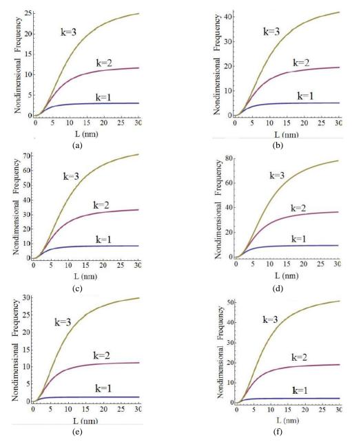
Fig. 4 Nondimensional frequency versus length for three frequencies modes in which scale coefficient
