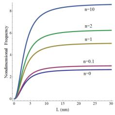
Fig. 16 Nondimensional frequency versus length for clamped-clamped boundary condition for the selected values of the n in power law function (k=1 and  $\mu=1$  nm)
