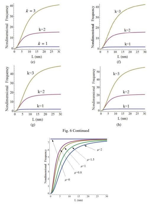
Fig. 7 Nondimensional frequency versus length with regard to different values for nonlocal parameter assumed for clamped-clamped FG nanobeam for power law
