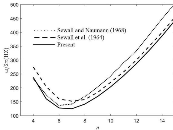
Fig. 3 Comparison of the natural frequencies of isotropic internal stiffened cylindrical shell ( $m = 1$ )
