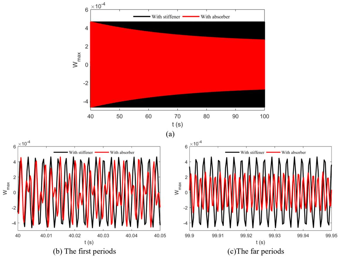
Fig. 4 Comparison of the effect of absorber without damper and stiffener on the vibration response of FG cylindrical shell
