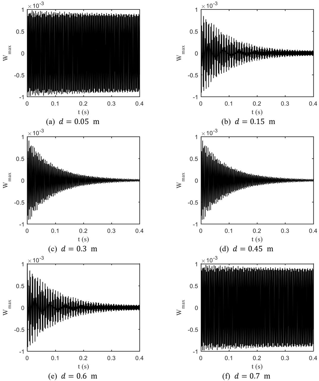
Fig. 9 The effect of vibration absorbers on the different places of FG cylindrical shell
