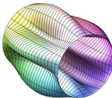
Fig. 5 The mode shapes of the FG cylindrical shell
