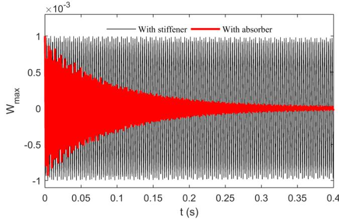
Fig. 6 The effect of absorber with local damper on the vibration response of FG cylindrical shell
