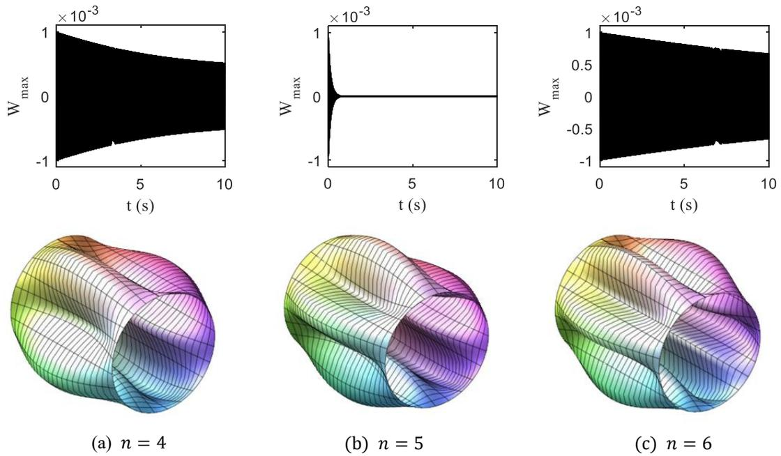
Fig. 12 The effect of different full wave ( $n$ ) on the vibration responses ( $m = 1$ )
