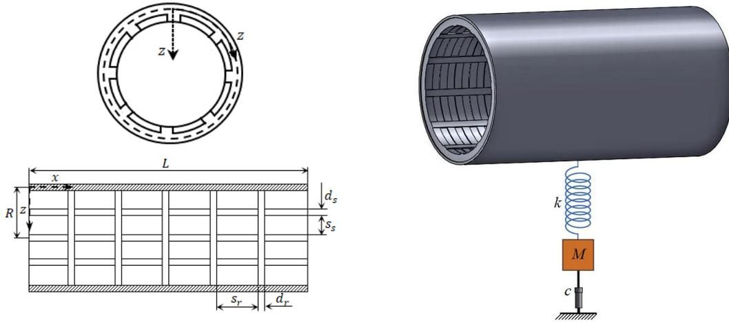
Fig. 1 Configuration of SFG cylindrical shell
