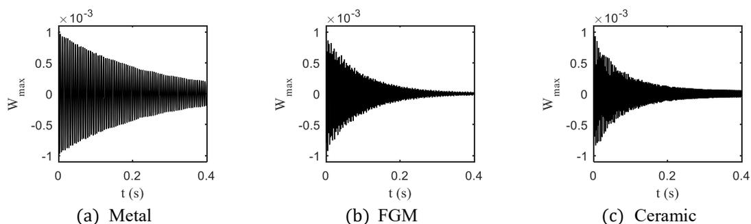
Fig. 10 The effect of material composition of FG cylindrical shell on the vibration responses
