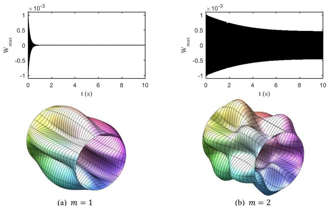
Fig. 11 The effect of different half waves ( $m$ ) on the vibration responses ( $n = 5$ )
