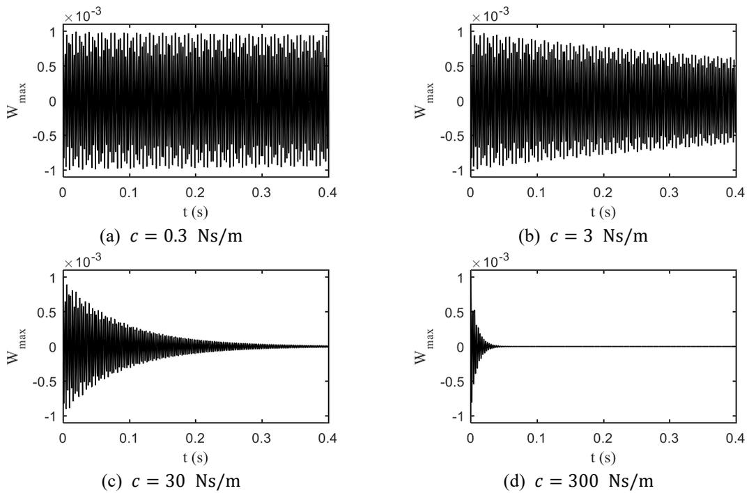
Fig. 8 The effect of various damping coefficients on the vibration responses of FG cylindrical shell
