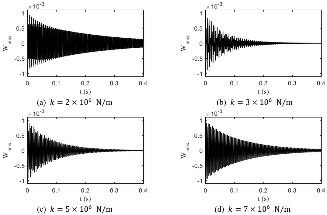
Fig. 7 The effect of different spring stiffness on the vibration responses of FG cylindrical shell
