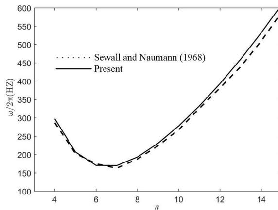
Fig. 2 Comparison of the natural frequencies of isotropic un-stiffened cylindrical shell ( $m = 1$ )
