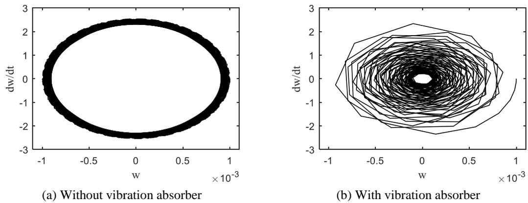
Fig. 13 Maximum deflection-velocity relation of FG cylindrical shell
