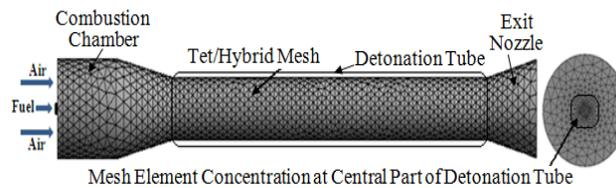
Fig. 2 Tet/Hybrid mesh generation and boundary details of computational domain
