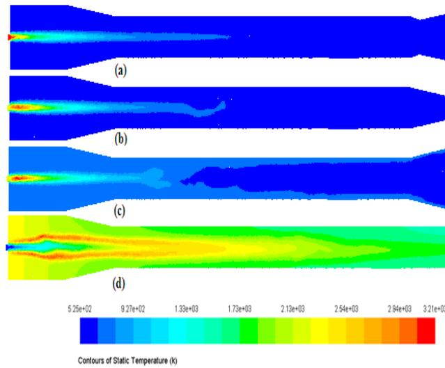
Fig. 4 Contour of static temperature of combustion wave
