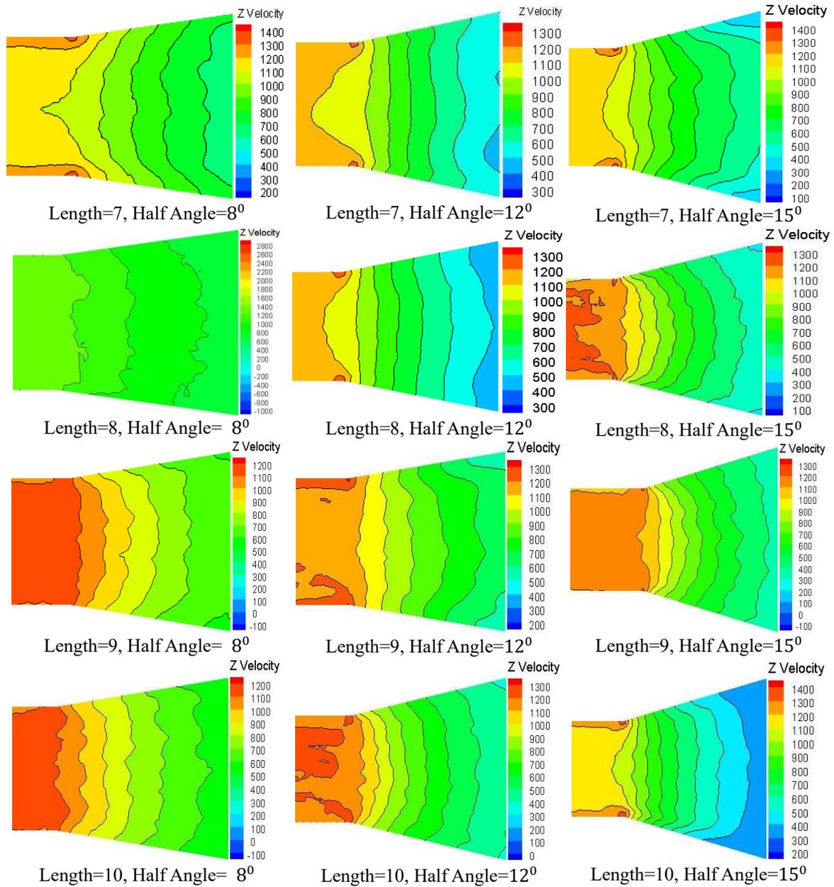
Fig. 13 Comparison of instantaneous detonation wave velocity flow field structure contour based on different half angle and nozzle length at a glance
