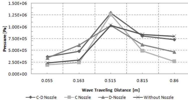
Fig. 11 Pressure distribution along the PDE combustor
