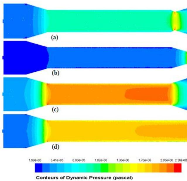
Fig. 5 Detonation wave dynamic pressure (Pascal) contours for (a) convergent divergent nozzle, (b) convergent nozzle, (c) divergent nozzle and (d) clean configuration
