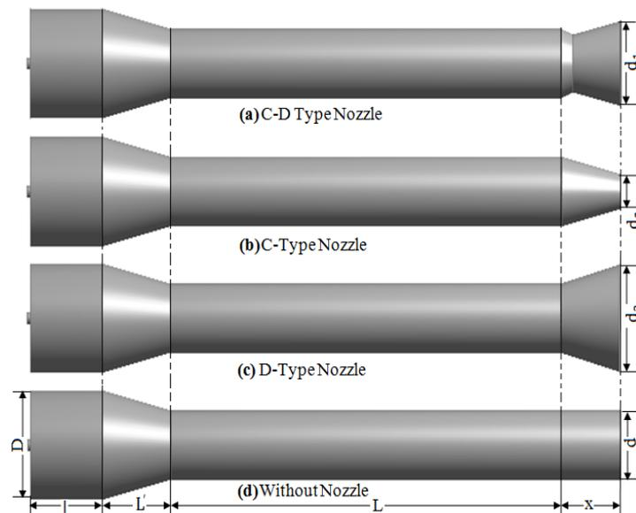
Fig. 1 Physical model of PDE with (a) convergent divergent nozzle, (b) convergent nozzle, (c) divergent nozzle and (d) clean configuration at exit section of detonation tube
