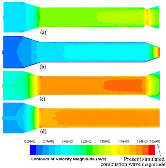
Fig. 6 Detonation wave velocity (m/s) magnitude contours for (a) convergent divergent nozzle, (b) convergent nozzle, (c) divergent nozzle and (d) clean configuration
