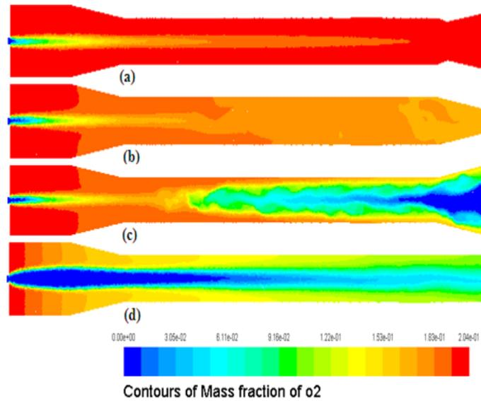
Fig. 8 Contour of  $O_2$  mass fraction of combustion product
