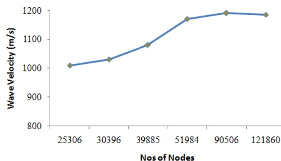
Fig. 3 Grid independence study of PDE with divergent nozzle
