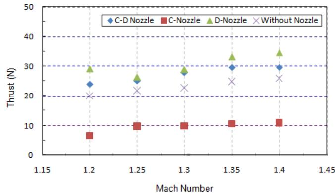
Fig. 12 The thrust variation for C-D nozzle, C-nozzle, D-nozzle and without nozzle configuration at different Mach number
