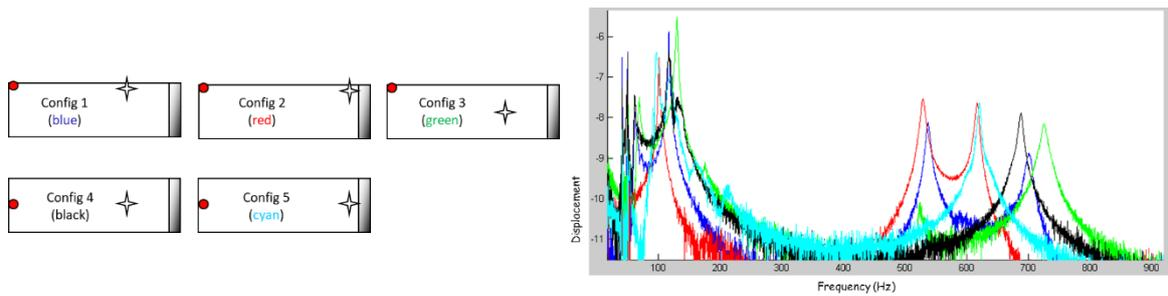
(a) Excitations (red discs) and measurements (stars) normal to the clamped (shaded area) panel (b) First few modes Fourier Transfer Functions (FTF) frequency responses
