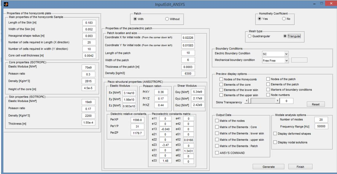
Fig. 14 The developed GUI for the free-vibration analysis of hexagonal honeycomb sandwich panels
