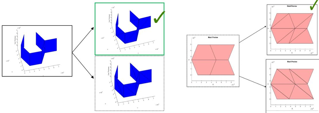
(a) Core hexagonal cell mesh triangularization (b) Face cell mesh triangularization
