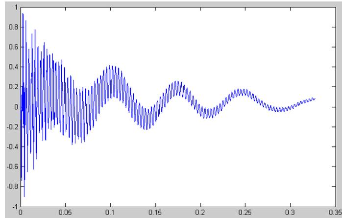
Fig. 3 Illustration of the high damping of the honeycomb sandwich panel (here simply-supported-SS; abscissa: time in s, ordinate: voltage in V)
