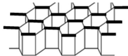
(a) Hexagonal cells geometric irregularities      (b) In-plane bonding double thickness walls (in bold)
