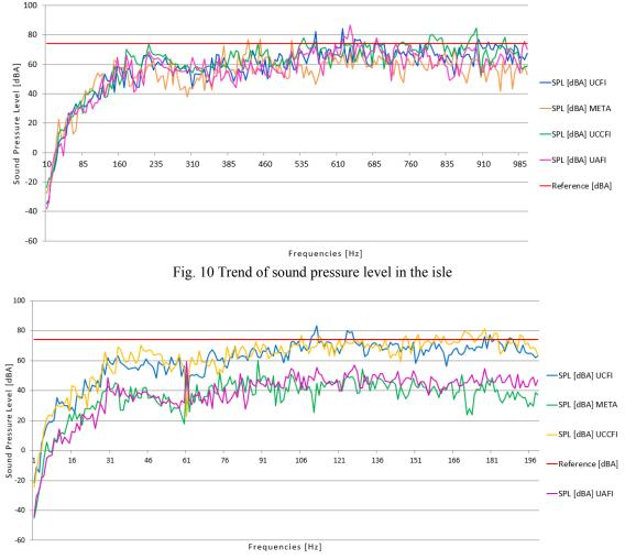
Fig. 11 Trend of sound pressure level at the ears of the window seat
