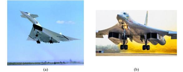
Fig. 1 Twin intakes used in jets: (a) North American XB – 70 Valkyrie (Wikipedia 2017), (b) Russian TU-160 Blackjack (Военное обозрение 2018)
