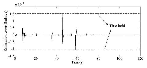
Fig. 4 The residual(estimation error) in a fault-free case obtained by SMO
