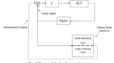
Fig. 3 Proposed fault tolerant scheme
