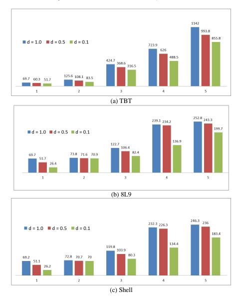
Fig. 12 Effect of the top flange damage level on the first five natural frequencies (Hz) of the I-beam via different models
