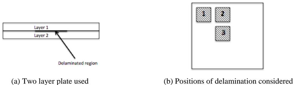
Fig. 2 Two layer laminated composite sandwich used and the positions of delamination considered
