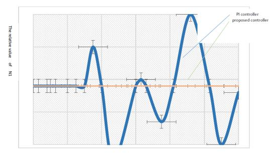
Fig. 1 The simulation results of harmonic disturbance of steady state power management particularly depicted low pressure rotor speed  $N_1$  versus time (s). Turbine outlet temperature versus time (s)
