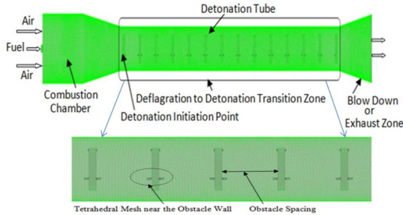
Fig. 2 Tetrahedral mesh of combustion domain with obstacles
