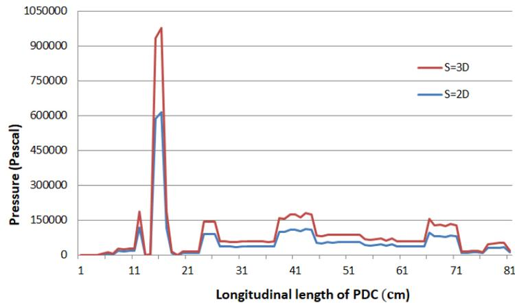
Fig. 11 Detonation wave pressure fluctuation at different wave traveling distance in detonation tube at pulse time of 0.031s
