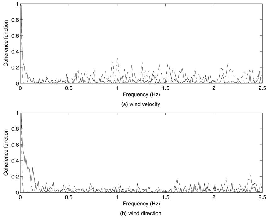
Fig. 6(a) Coherence between wind speed and direction at 30 m and 50 m levels ( — typhoon, - - - weak wind)
