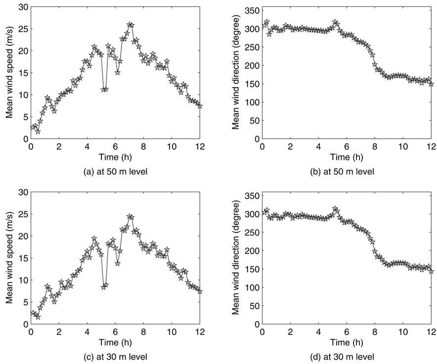
Fig. 3(b) 10-minute mean wind speed and direction (from 14:00 2nd Sept. to 02:00 3rd Sept.)
