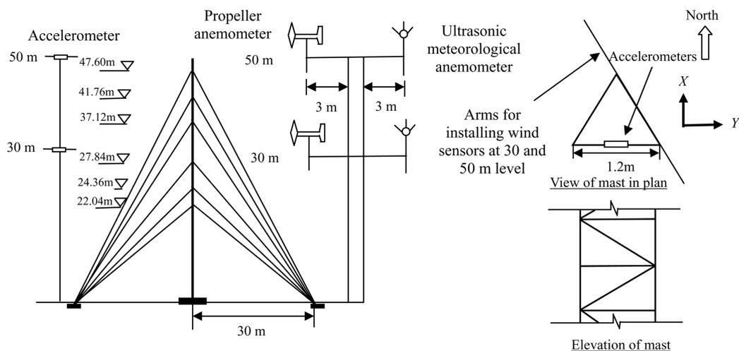
Fig. 1 Schematic view of the instrumented guyed mast
