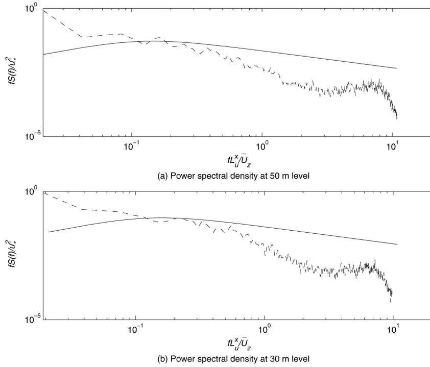
Fig. 5(b) Power spectral density of weak wind at 30 m and 50 m levels ( — von Karman, - - - measured)
