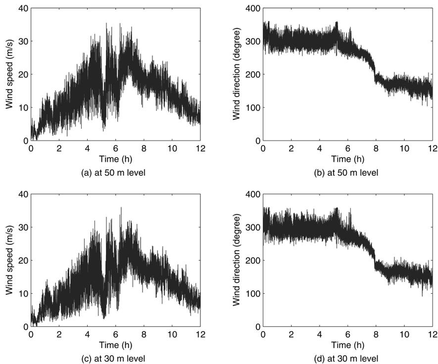
Fig. 3(a) Measured wind speed and direction for 12 hours (from 14:00 2 Sept. to 02:00 3 Sept.)
