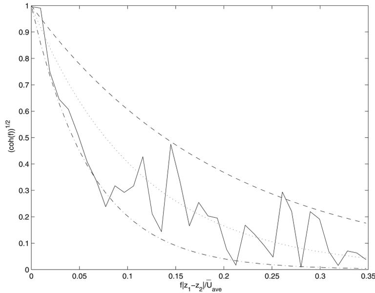
Fig. 6(b) Davenport's coherence between wind speed at 30 m and 50 m levels ( — measured, - - -  $C_z=5$ , ····  $C_z=8$ , - · - ·  $C_z=15$ )
