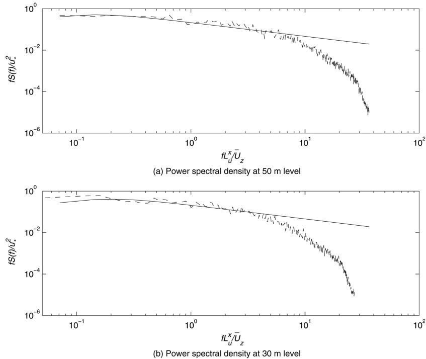
Fig. 5(a) Power spectral density of typhoon at 30 m and 50 m levels ( — von Karman, - - - measured)
