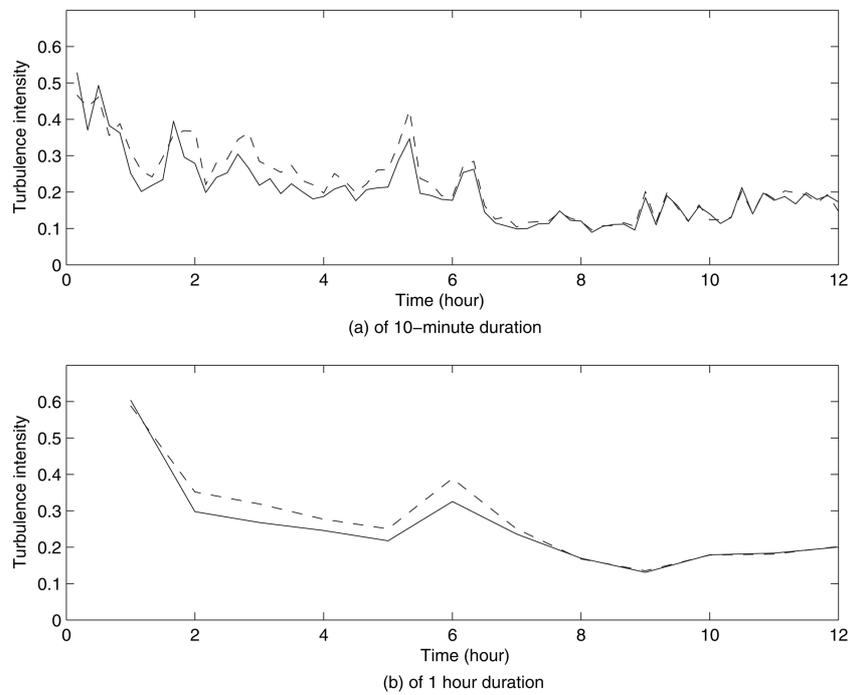
Fig. 4 Turbulence intensity of 10-minute and one hour duration ( — at 50m level, - - - at 30m level)
