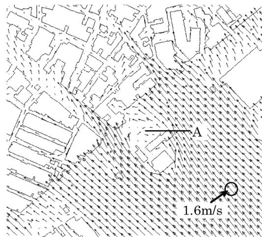
Fig. 12 Horizontal wind velocity vector distribution around the crossing (Case 3, height: 1.5 m)
