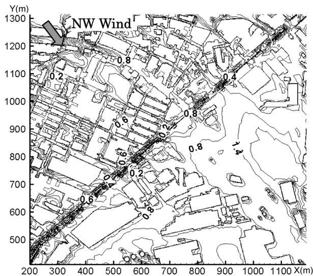
Fig. 8 Horizontal wind velocity scalar distribution in the whole area (Case 2, height: 1.5 m)
