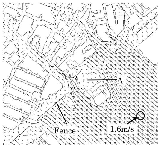
Fig. 10 Horizontal wind velocity vector distribution around the crossing (Case 1, height: 1.5 m)
