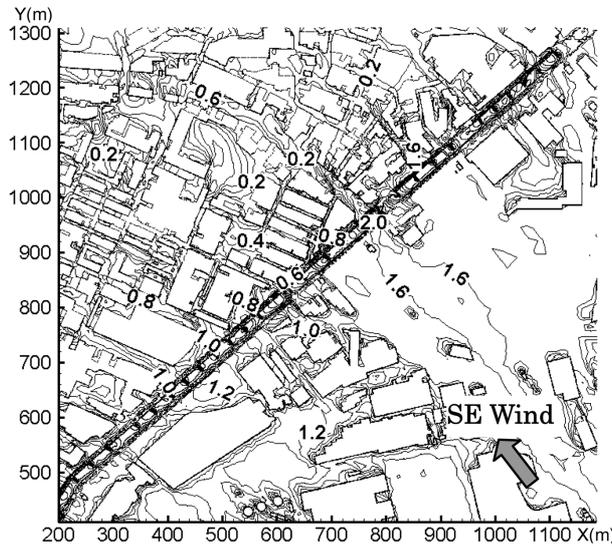
Fig. 9 Horizontal wind velocity scalar distribution in the whole area (Case 3, height: 1.5 m)
