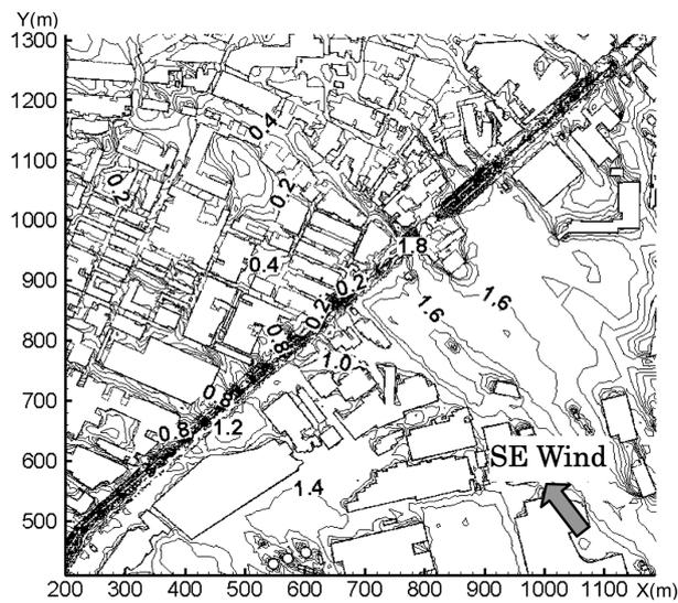
Fig. 7 Horizontal wind velocity scalar distribution in the whole area (Case 1, height: 1.5 m)
