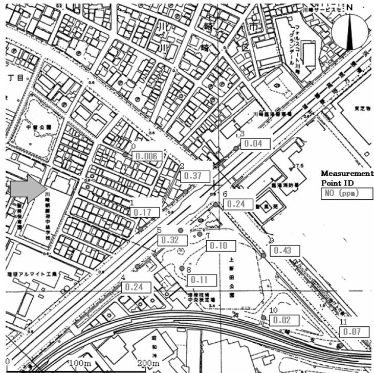
Fig. 3 NO concentration at each point at 11:00 of the field measurement
