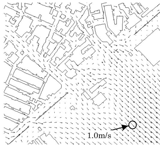
Fig. 11 Horizontal wind velocity vector distribution around the crossing (Case 2, height: 1.5 m)
