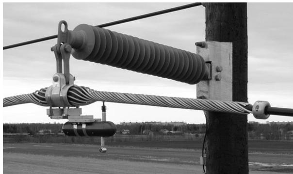
Fig. 11 Vibration recorder installed below AGS-clamp
