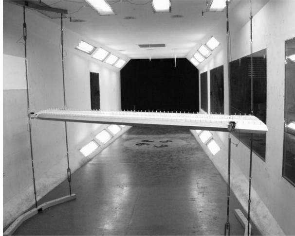
Fig. 5 Test model for flutter derivative measurement
