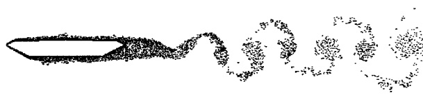
Fig. 3 Vortex shedding from static Storeboelt Bridge, instantaneous vorticity field from DVM
