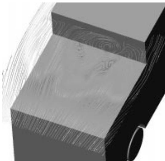
Fig. 3 Output from PowerFLOW showing asymmetric streamlines above the cab
