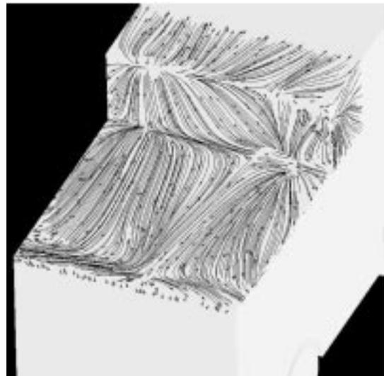
Fig. 4 Output from PowerFLOW showing asymmetric surface flow on the cab and trailer front
