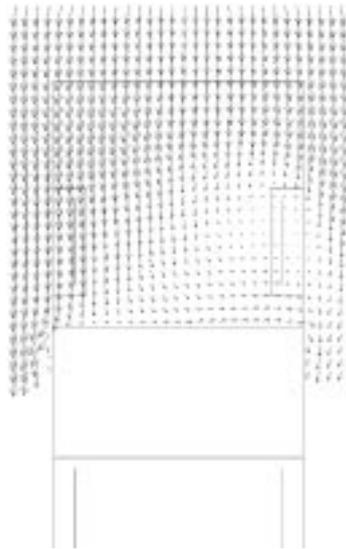
Fig. 2 Output from CFX showing asymmetry across lorry cab. (Flow enters from the top; arrows represent velocity vectors; flow is displayed on a plane parallel with the ground, above the cab surface.)
