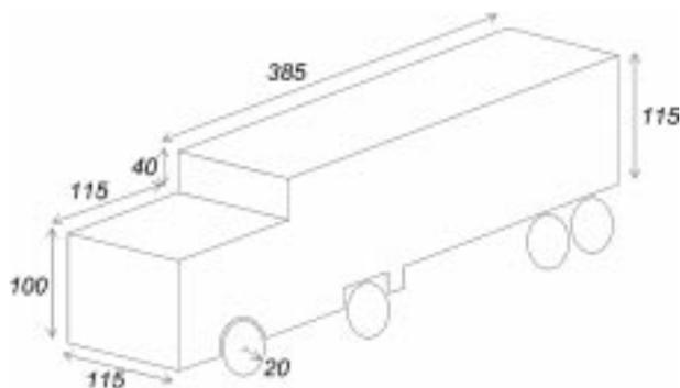
Fig. 1 Schematic representation of the lorry (Dimensions in mm. Not to scale)
