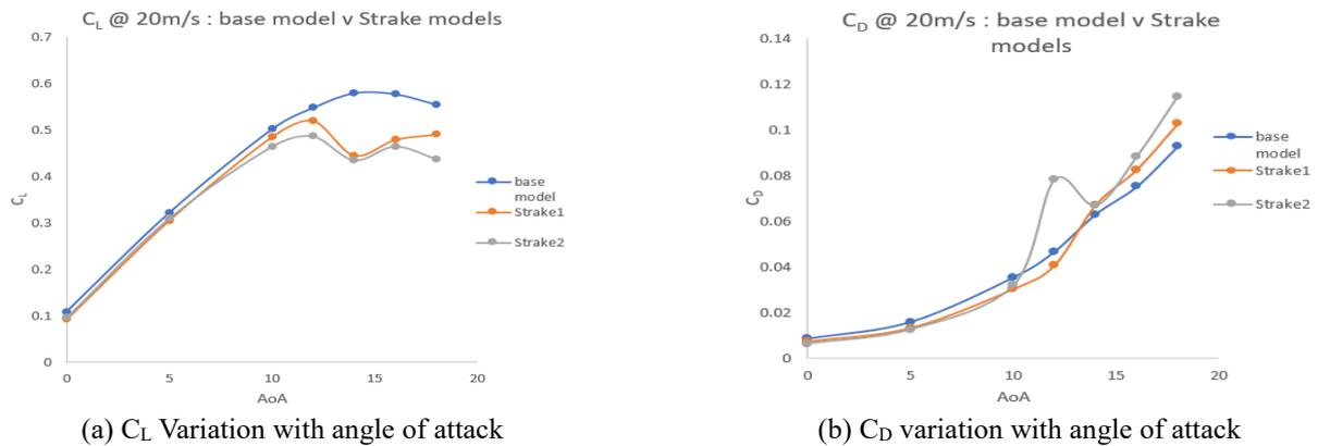
Fig. 6. Aerodynamic performance of Base wing and wing with leading edge strake
