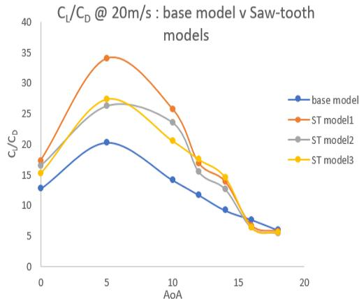
Fig. 7 Aerodynamic efficiency (L/D) variation with angle of attack
