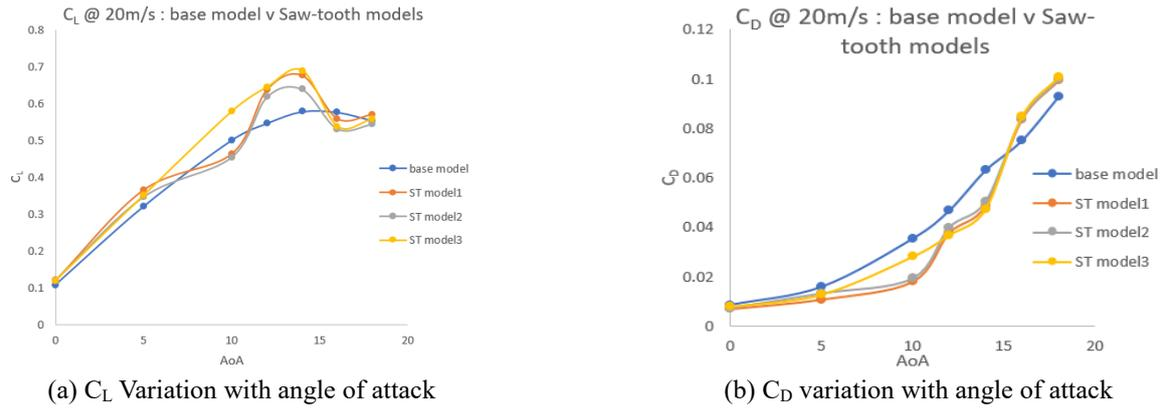
Fig. 5. Aerodynamic performance of Base wing and wing with saw-tooth
