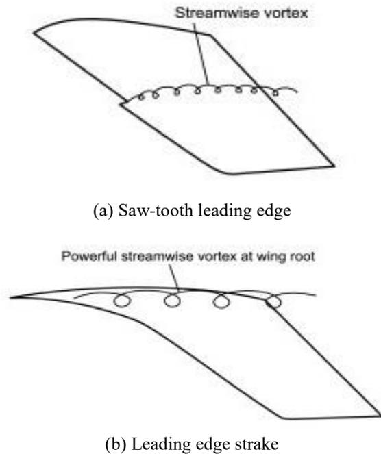
Fig. 1 Passive vortex generators (Houghton et al. 2012)
