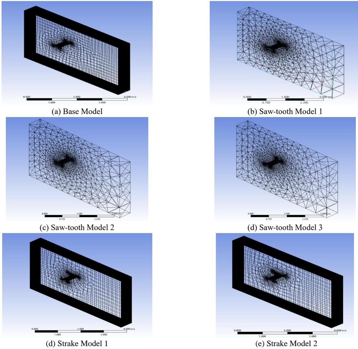
Fig. 3 Meshed wing base model and models with modification
