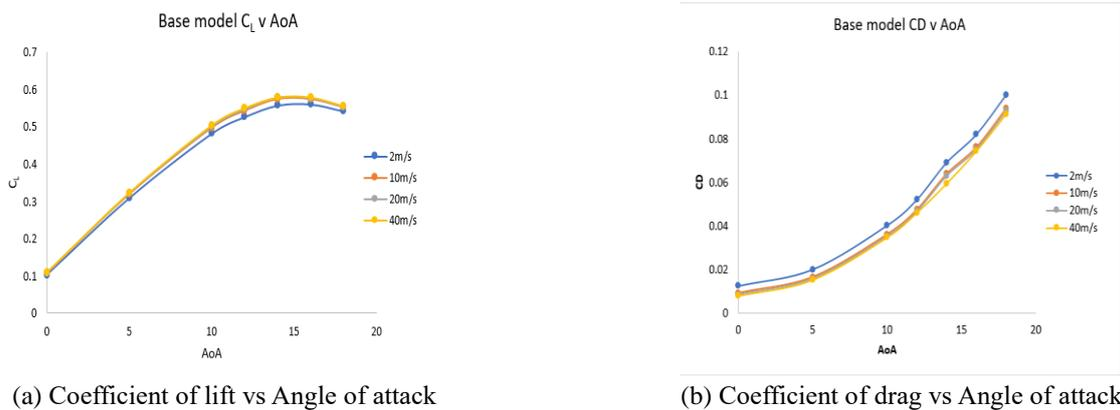
Fig. 4 Aerodynamic performance of the Base model wing
