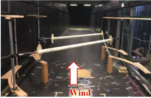
Fig. 5 Test setup of yawed grooved cylinders in tandem arrangement
