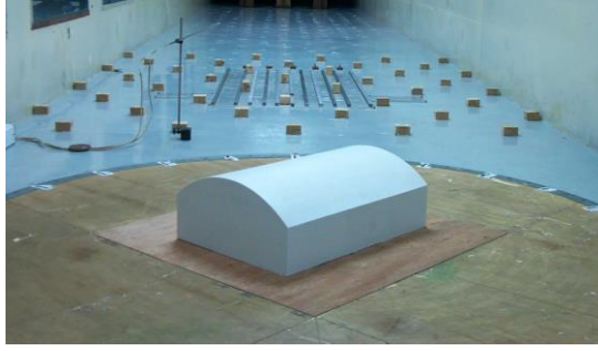
Fig. 1 Wind tunnel model of the structure
