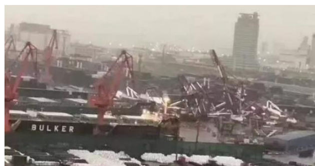
Fig. 1 Five quayside container cranes were blown down by a strong transient gusty wind (Qingdao Port 2018)
