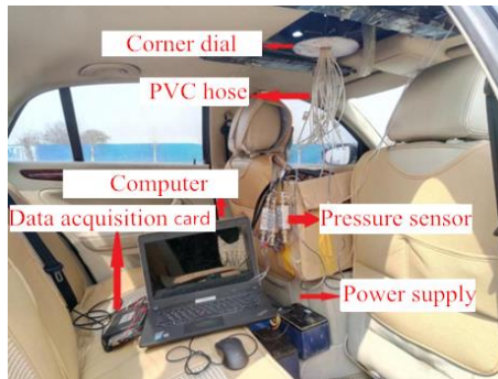
Fig. 2 Interior collecting instrument and system arrangement
