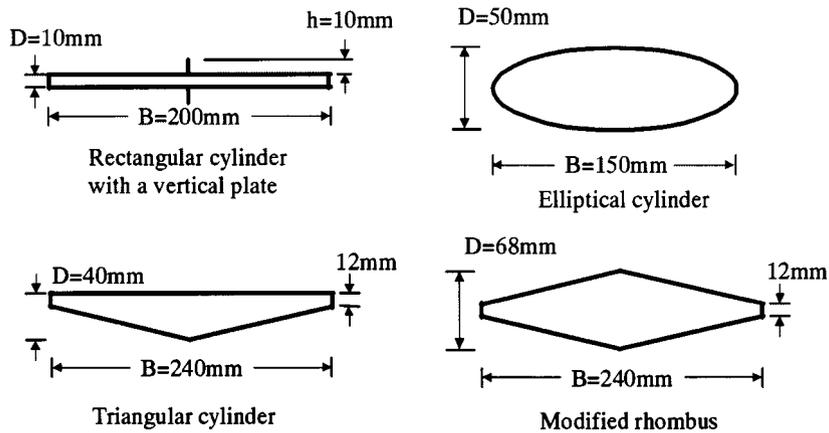
Fig. 9 Comparatively stable isolated deck sections against flutter instability
