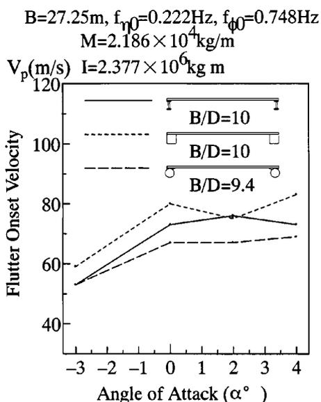
Fig. 5 Flutter instability depending on the edge girder shape and the angle of attack of wind
