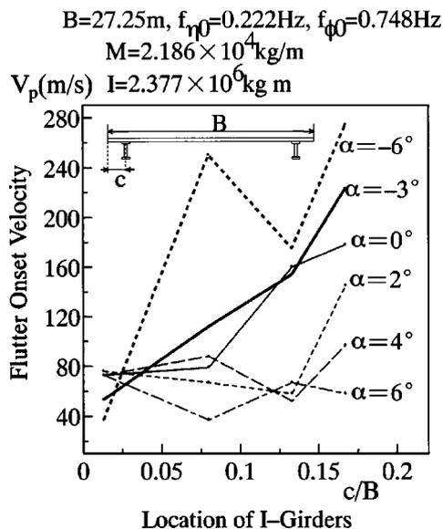
Fig. 6 Flutter instability depending on the location of edge girders and the angle of attack of wind
