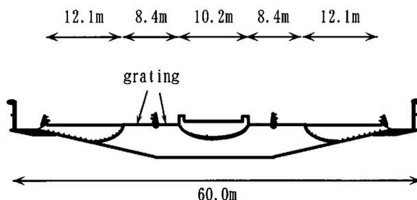
Fig. 8 Deck cross section of the Messina Straits Bridge
