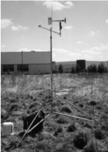
Fig. 1 Portable near-ground wind station with anemometer at a 3 m (10 ft) height above ground
