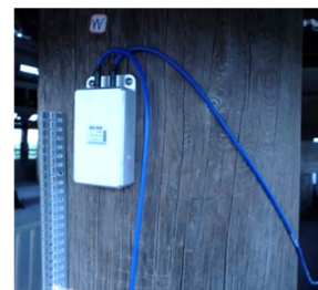
(a) FBG inclination sensor on the top of the column
