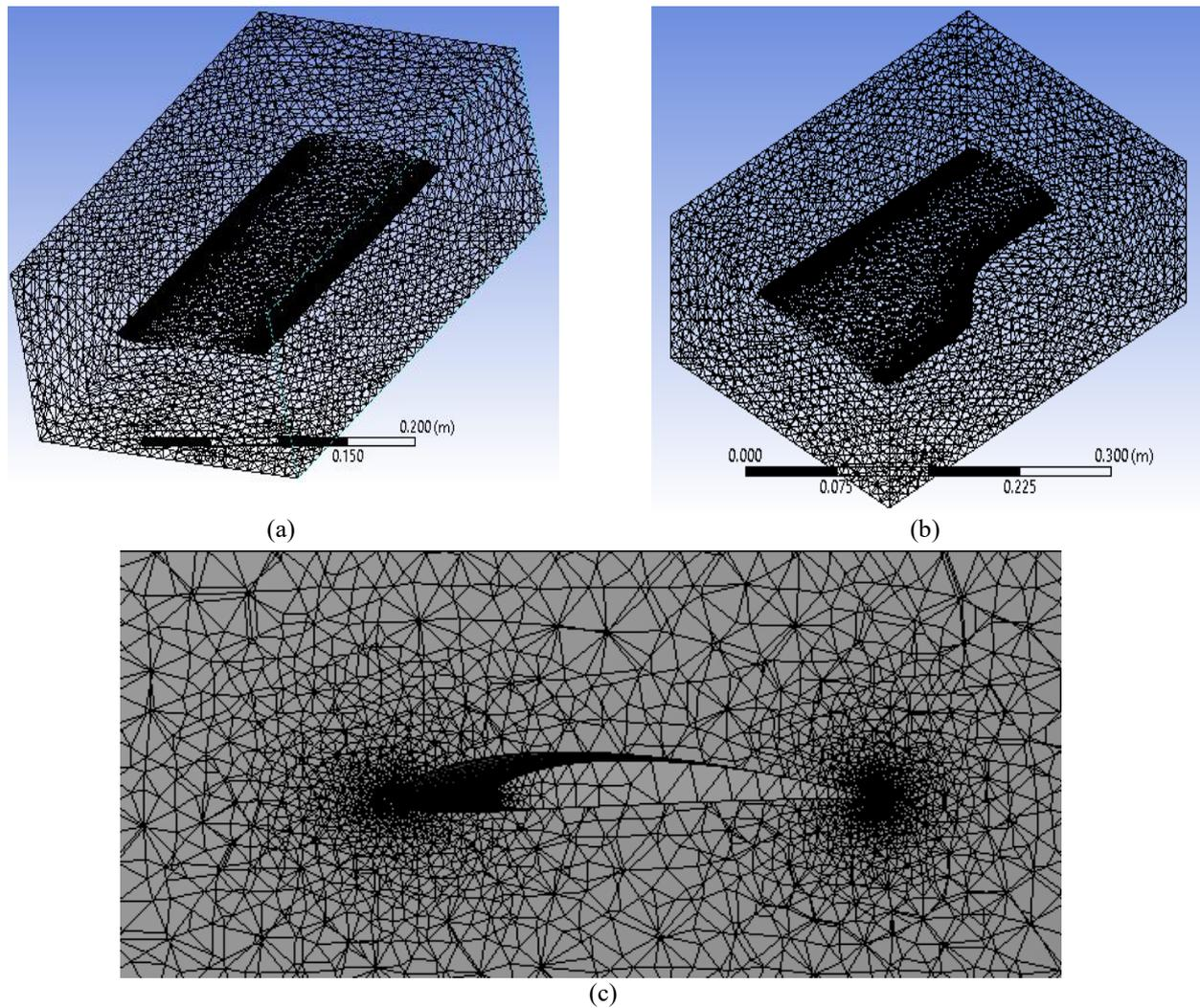
Fig. 2 (a) Meshed rectangular wing, (b) Meshed wing with a curved leading edge and (c) Cut sectional view of the wing
