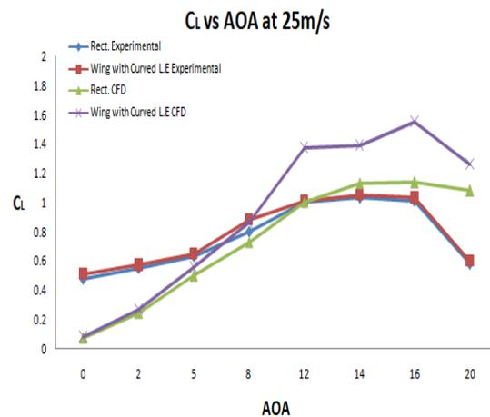
Fig. 5 Comparison of the coefficient of lift at various angles of attack
