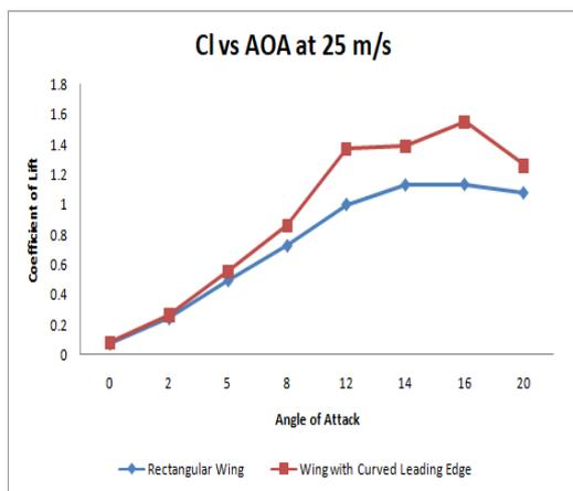
Fig. 3 Variation of the coefficient of lift with angles of attack
