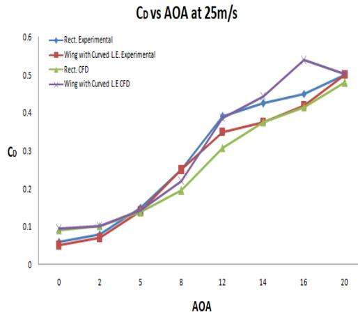
Fig. 6 Comparison of the coefficient of drag at various angles of attack
