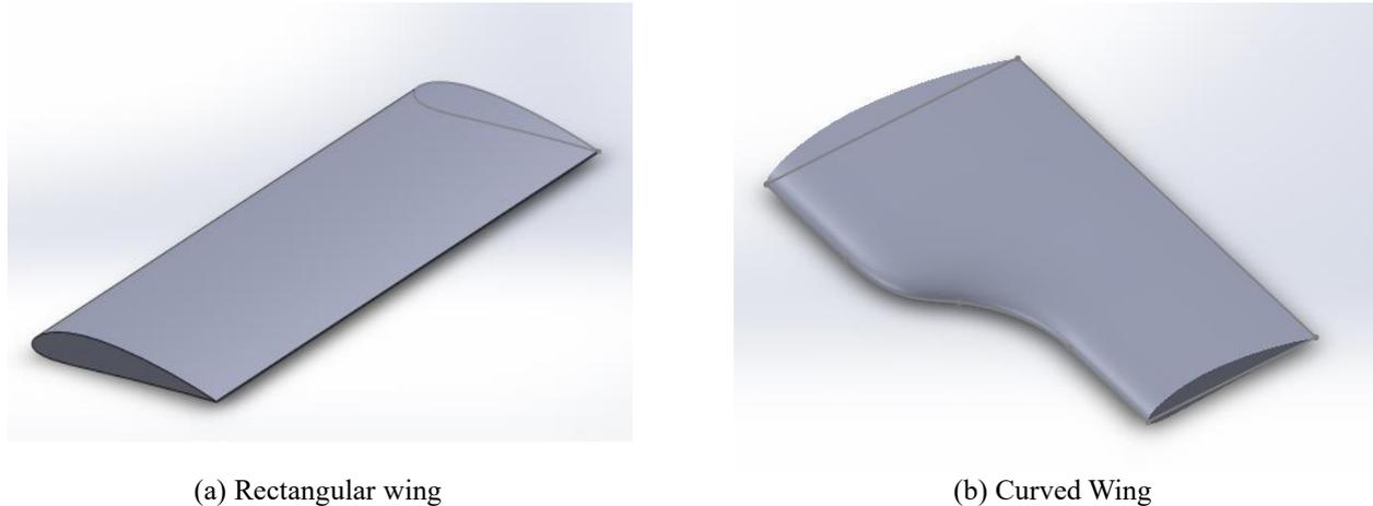
Fig. 1 Wing model for rectangular and curved leading Edge Planforms
