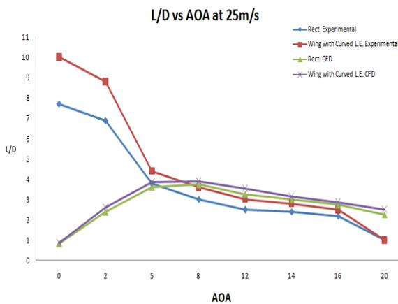
Fig. 9 Aerodynamic efficiency (L/D) variation with angles of attack
