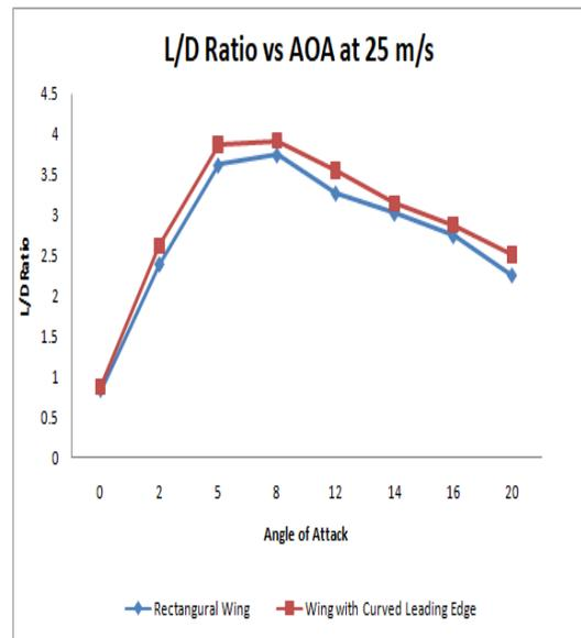
Fig. 4 Variation of lift to drag ratio(aerodynamic efficiency) with angles of attack
