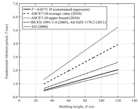
Fig. 13 Comparison of the proposed formula for fundamental vibration period versus building height for RC frame-shear wall buildings with those in the design codes and standards
