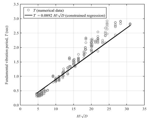
Fig. 6 Fundamental vibration period versus height and plan dimensions of RC frame-shear wall buildings with constrained regression formula
