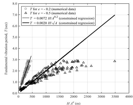
Fig. 10 Fundamental vibration period versus building height and effective shear area ratio for RC frame-shear wall buildings with constrained regression formulas
