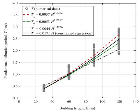
Fig. 4 Fundamental vibration periods versus building height for RC frame-shear wall buildings with AR = 1:1 to 1:2
