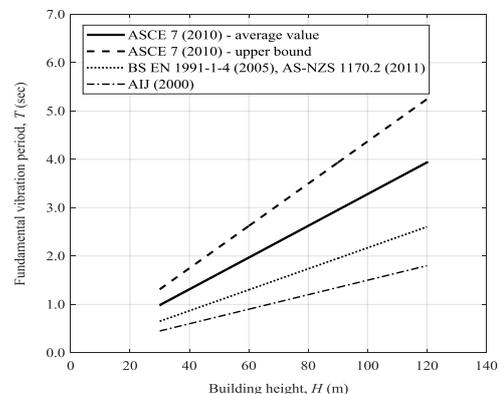
Fig. 1 Fundamental vibration period versus building height in the design codes and standards
