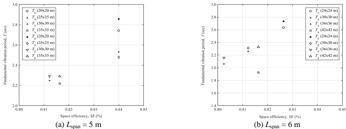
Fig. 11 Fundamental vibration period versus space efficiency for 40-storey buildings with AR = 1:1
