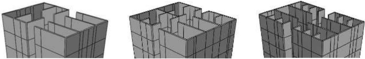
Fig. 3 Typical plan configurations for the cores of RC frame-shear wall office building models
