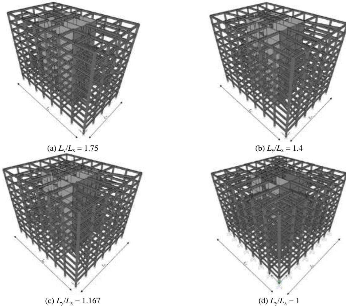
Fig. 2 3-D views of ten-storey RC frame-shear wall office building models with various plan aspect ratios
