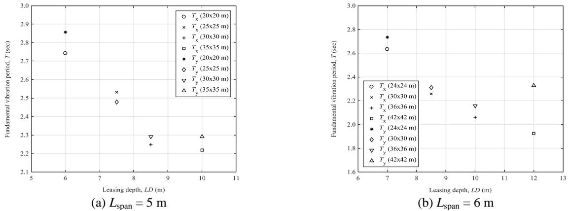
Fig. 12 Fundamental vibration period versus leasing depth for 40-storey buildings with AR = 1:1
