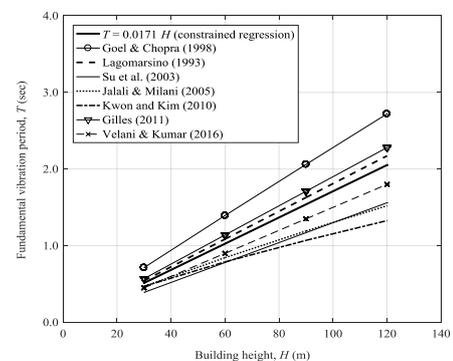
Fig. 14 Comparison of the proposed formula for fundamental vibration period versus building height for RC frame-shear wall buildings with those from the prior experimental studies
