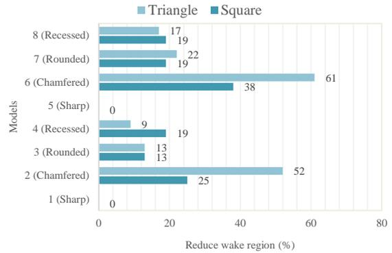
Fig. 6 Wake region reduction in the models with square and triangular footprints comparing to reference Sharp models T1 and S1
