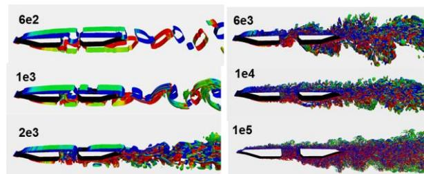
Fig. 7 Vortex structures at  $Re = 6e3, 1e4, 1e5$  ( $\lambda_2 = -0.1$ , the vortex structures are colored by  $z$ -vorticity with the range of  $[-10, 10]$ )
