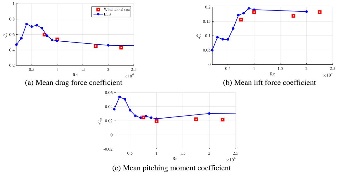
Fig. 4 Comparison of the aerodynamic forces and vortex shedding frequency obtained by LES and experiments
