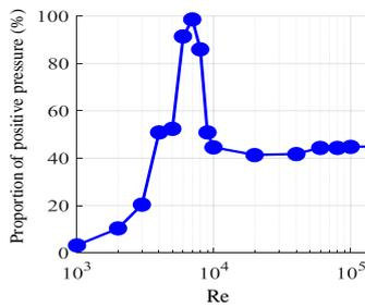
Fig. 13 Relationship between the proportion of positive pressures on the downstream wall of the gap and the Reynolds number
