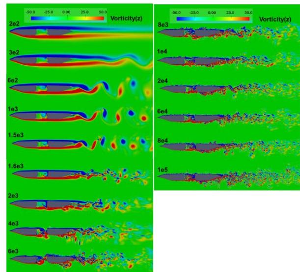
Fig. 6 Instantaneous  $z$ -direction ( $z/D = 0.5$ ) vorticity contours at various Reynolds number
