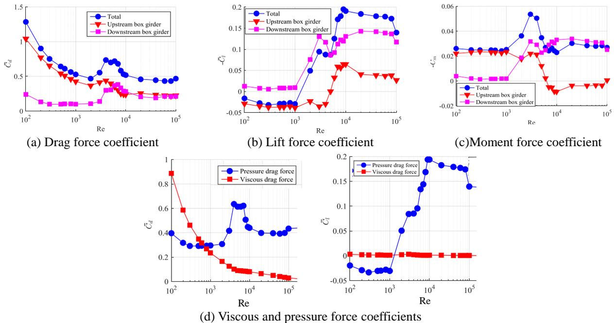
Fig. 15 Relationship between mean aerodynamic force coefficients and the Reynolds number
