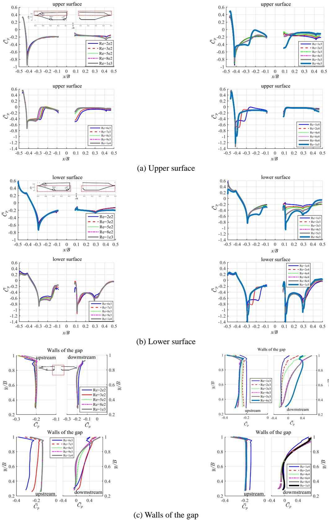
Fig. 8 Mean pressure distributions on the surface of twin-box girder at various Reynolds numbers
