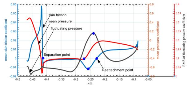
Fig. 10 Mean skin-friction coefficient on the upper surface of upstream box girder at  $Re=6e3$
