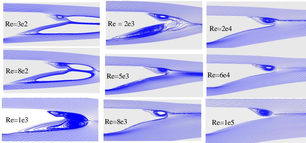
Fig. 14 Mean streamlines around the trailing edges at various Reynolds numbers
