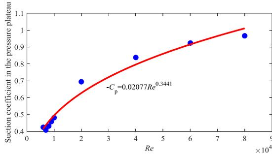
Fig. 12 Relationship between the suction coefficient of pressure plateau and the Reynolds number
