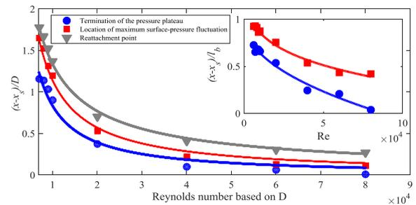
Fig. 11 Termination of the pressure plateau and the location of the maximum surface-pressure fluctuation against the Reynolds number ( $x_s$  is x-direction location of separation point,  $l_b$  is bubble length)
