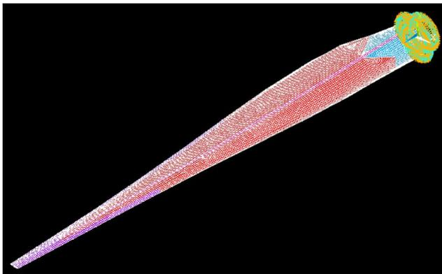
Fig. 11 Constraints on the blade FEM model
