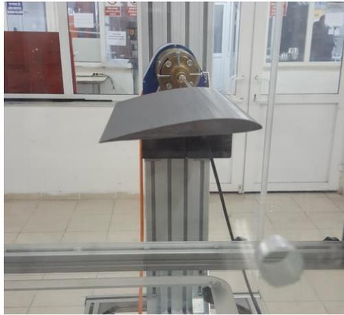
Fig. 14 A18 airfoil in the test area of wind tunnel
