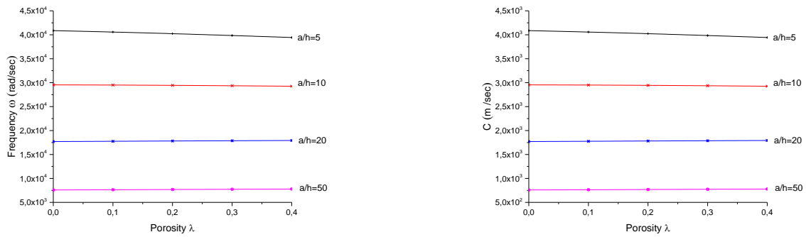
Fig. 8 Influence of the porosity on the natural frequency and phase velocity of the different plates
