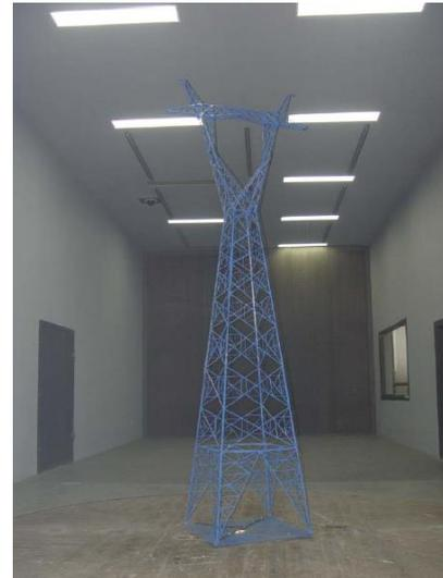
Fig. 2 Rigid tower model in wind tunnel
