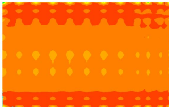
(c) Stress in y direction, maximum=111083.41 \text{KN/m}^2 (fixed connection)
