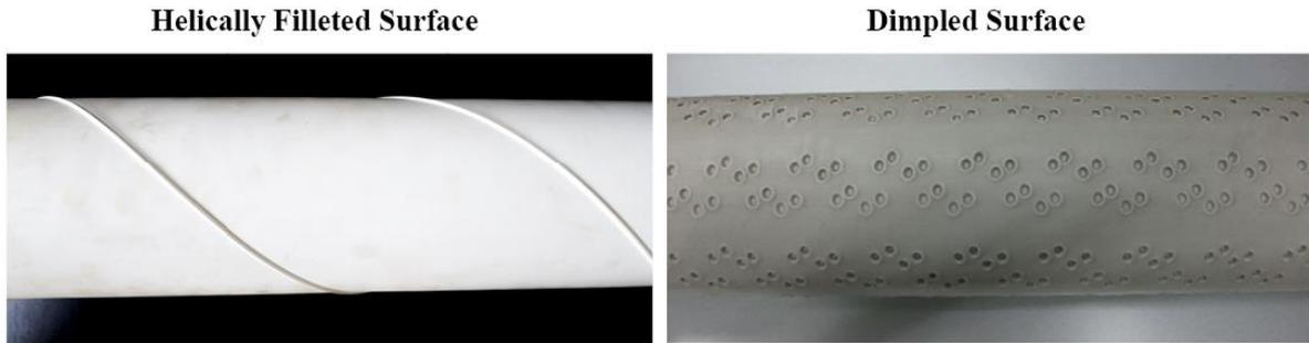
Fig. 1 Cable sample models from previous aerodynamic measures
