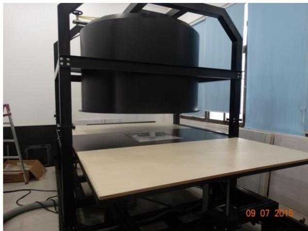
Fig. 2 Experimental Setup-Tornado Like flow Simulator at Tongji University
