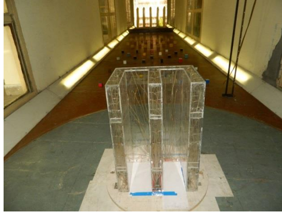
Fig. 3 Model placed inside wind tunnel
