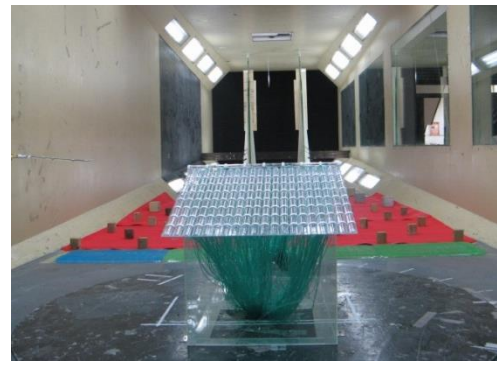
(b) Concrete tile roof
