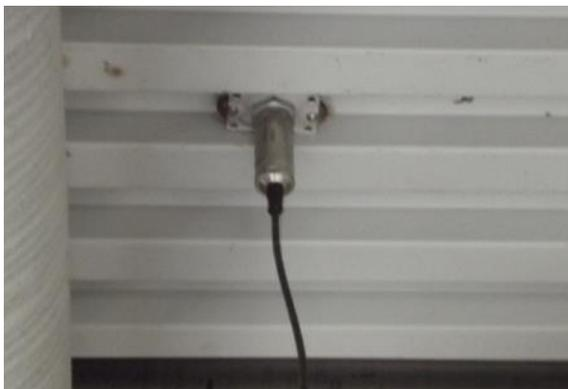
Fig. 4 wind-pressure transducer
