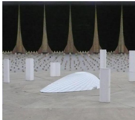
Fig. 1 Rigid model for wind tunnel tests
