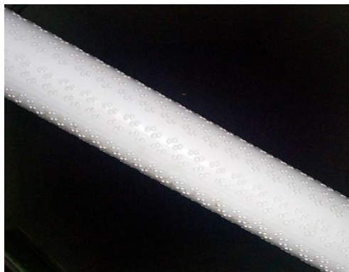
Fig. 2 Cable model with dimpled pattern on the surface
