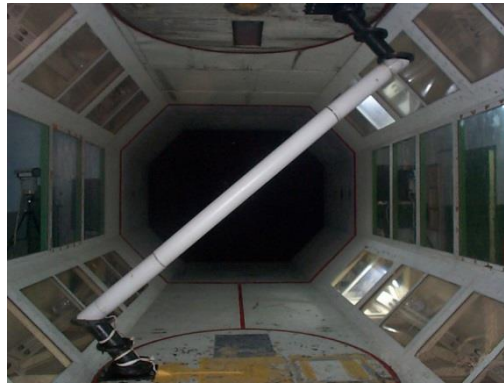
Fig. 5 Installation of the model system in the wind tunnel
