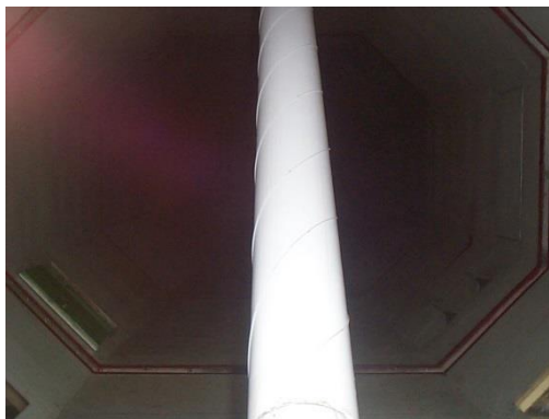
Fig. 3 Cable model with 2 mm helical fillet on the surface
