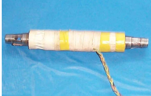
Fig. 4 TG0401 balance used for measuring the wind force acting on the circular cylinder
